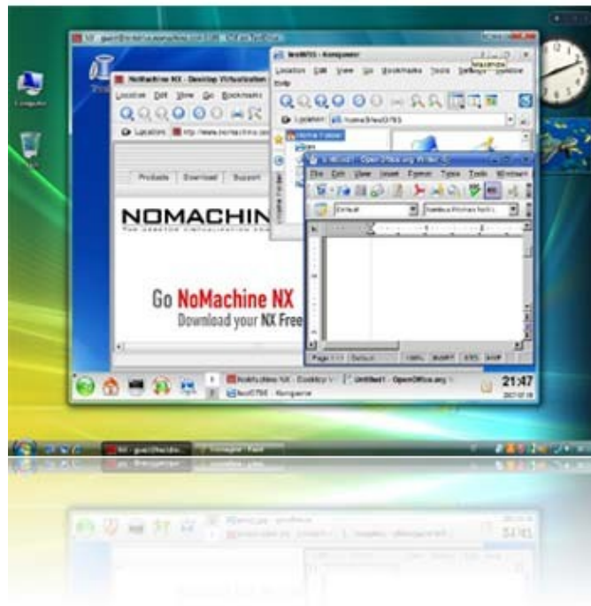
Fig 1. A remote KDE session displayed on a local Windows Vista desktop using the NX Client for Windows.
